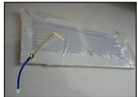
Figure 17: A Static Pressure Probe attached to a pressure tube allows the measurement of pressure without flow interference (e.g. inside a supply register)
