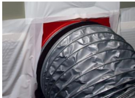
Figure 18: Flex Duct connected to the Flange.
