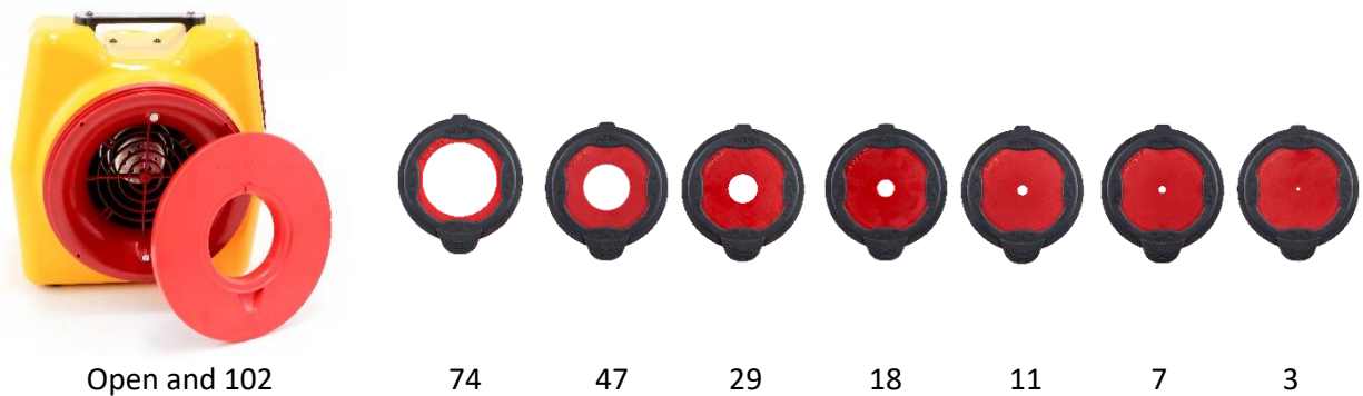
Figure 3: Range 102 is for the leakiest ducts while the smaller ranges are for progressively tighter ducts.
