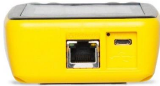
Figure 14: Electrical connections on the bottom of the gauge include Network (Ethernet) Cable that goes from the DM32 to a PC (if Retrotec PC software is used for data collection), micro USB cable for PC software and/or charging, and a reset button.
