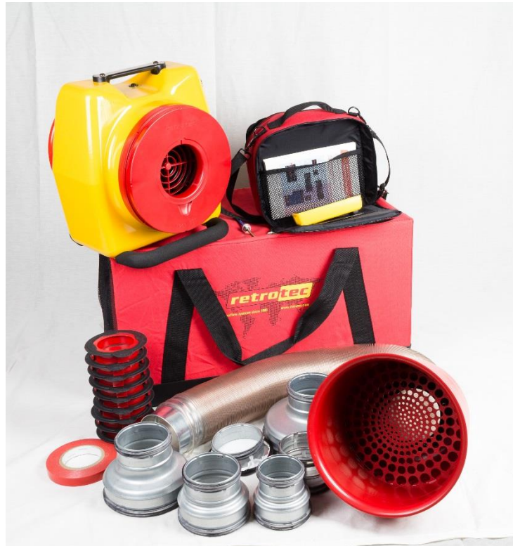
Figure 2: A complete duct testing system.
