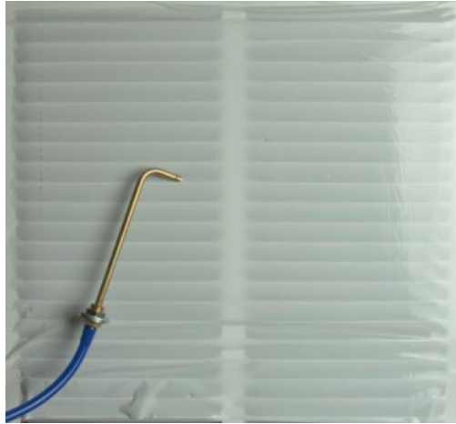
Figure 16: Insert the blue tube into a supply register closest to the air handler
