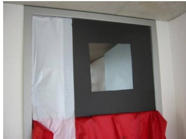
Figure 18: Homemade verification plate.
