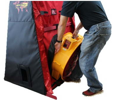
Figure 11: Installing a fan in the cloth door panel.
