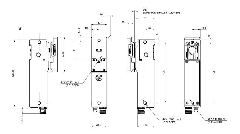
**ATOM** has a High-Coded RFID technology that provides millions of different coding combinations and is classed as "high" coding by ISO 14119.
