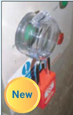
Designed to fit over push button switches to prevent accidental operation. Overall 50mm dia. with 30mm dia. hole. Secured with padlock - max. shackle dia. 7mm.
