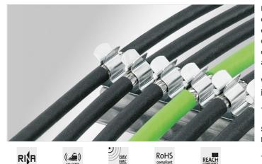
EMC clamp assemblies are used, where the shield of several cables must be connected to the earth potential. They are easy to use and enable effective earthing and strain relief of up to 12 cables in a small space. There are different carriers available which can be user configured with up to 12 SKL or MSKL shield clamps. The shield clamps are mounted directly on the surface of the clamp assembly which guarantees a tight fit.
