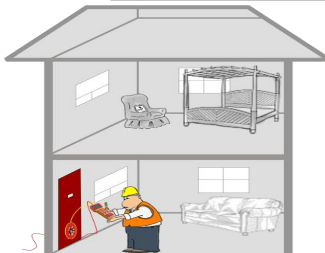
Figure 5: A Blower Door can be used to measure whole house leakage from any exterior doorway.
