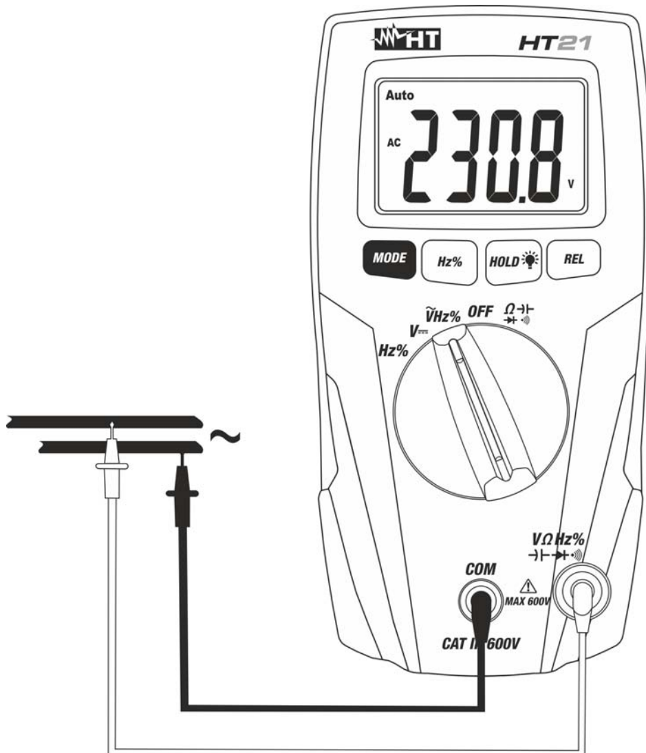
Fig. 3: Using the instrument for AC Voltage measurement
