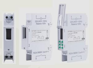
OP-DIN IS A SINGLE-MODULE DIGITAL DIN-RAIL TIMER, WITH L.C.D. AND 7 DAY / 24 HOUR PROGRAMMING CAPABILITY. THERE ARE 6 ON AND 6 OFF PROGRAMME SPACES. THE TIMER HAS A RE-CHARGEABLE CELL PROVIDING BATTERY BACK-UP OF TIME AND PRO-GRAMME IN THE EVENT OF MAINS FAILURE.
