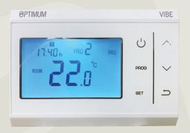
THE OPTIMUM VIBE - MODEL OP-HWSTAT IS A BATTERY POWERED PROGRAMMABLE ROOM THERMOSTAT WITH TOUCH-SCREEN STYLE CAPACITIVE CONTROLS, PROVIDING SIX TIMED TEMPERATURE PERIODS EVERY 24 HOURS. THE HWSTAT IS PROVIDED WITH A WALL-MOUNTING BACKPLATE AND INCORPORATES VOLT-FREE SWITCHING TERMINALS. IT HAS A LARGE BLUE BACKLIT DISPLAY AND RUNS A PRE-PROGRAMMED USER ADJUSTABLE TEMPER-ATURE PROFILE. USERS CAN JUST TOUCH THE UP OR DOWN CONTROL ICON AT ANY TIME TO MANUALLY ADJUST THE CURRENT TEMPERATURE SETTING.
