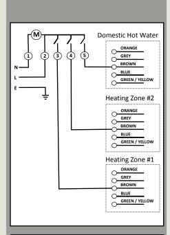
Connections for SBWF03: Controlling 2 heating zones and domestic hot water using 3 x 2-port zone valves
