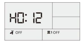
Press and hold [HOLIDAY ON/OFF] button for 3seconds to deactivate, when the holiday mode is activated. The programmer returns to normal mode.
