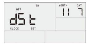
Daylight saving time is set to OFF DST symbol disappears.
