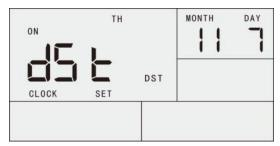
Daylight saving time is set to ON DST symbol displays.
