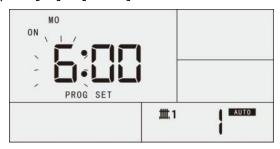
Press [SELECT] to set Channel 1 Monday P1-OFF. Press [UP] or [DOWN] to set hour. Then press [SELECT] and press [UP] or [DOWN] to set minute.
