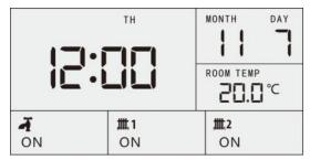
Operating mode: HW:ON C1:ON C2:ON
