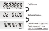
After the self-checking program, the meter display will show the total active energy (kWh)
