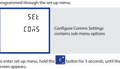
To enter set-up menu, hold the button for 3 seconds, until the screen appears.
