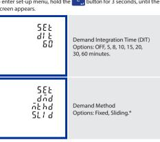
\* The Demand Method can be configued as follows: Sliding =  $0\sim60$  minutes,  $1\sim61$  minutes,  $2\sim62$  minutes etc Fixed =  $0\sim60$  minutes,  $60\sim120$  minutes,  $120\sim180$  minutes etc
