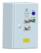
A solid state Time Delay unit for use where machines do not come to an immediate stop. The gate access key is held captive in the unit until the desired condition of the machine or process has been achieved. The time delay is internally programmable with range from 60 to 600 seconds (10 minutes). As part of an interlock system, the units are used to control keys giving access to enclosed areas or machines where hazards may be present, until a safe condition has been achieved.
