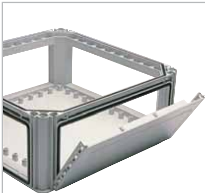
End-plates, combi or blind, are snapped on from the outside and fixed by means of vertically sunk keys.
